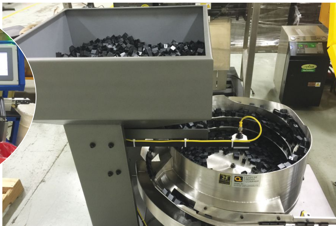
In D&M's factory, an automated optical sorting machine helps identify defective parts.
