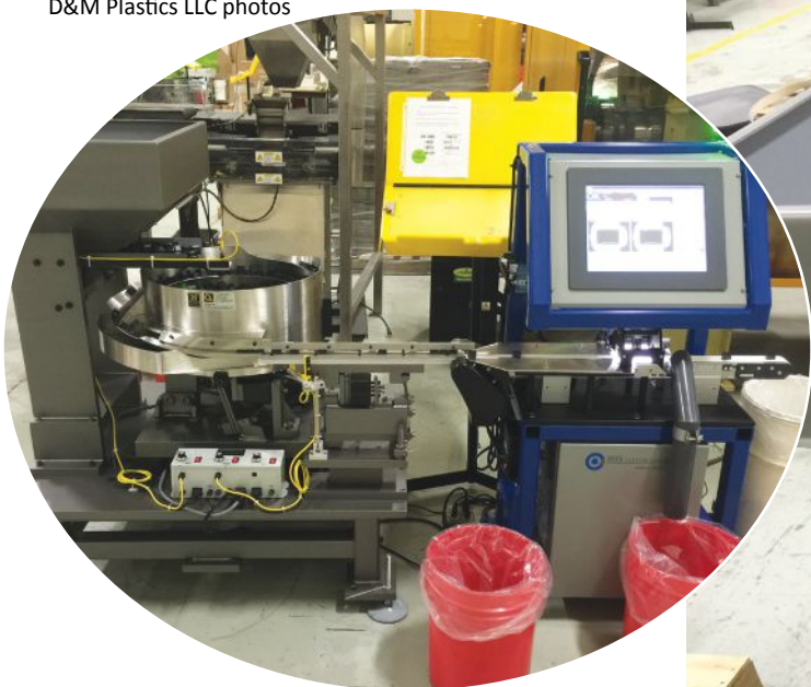
In D&M's factory, an automated optical sorting machine helps identify defective parts.
