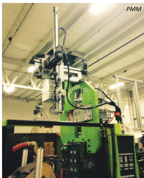
A robot is used in D&M's in-mold labeling process. The robot was customized for use on a 200-ton Engel horizontal press.
